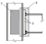
Joint = web panel in shear + connection 1 - web panel in shear 2 - connection 3 - components (e.g. bolts, endplate)
