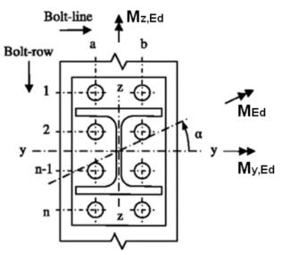
The strong-axis moment resistance  $M_{j,y,Rd}$  of the joint is determined based on EN 1993-1-8, assuming no weak-axis bending influence. Similarly to this, it is assumed that the strong-axis moment bending will not influence calculation of weak-axis moment resistance  $M_{j,z,Rd}$  of the joint.
