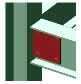
The bolt holes are not taken into account when:  $A_{v,net} \ge \frac{f_y}{f_u} \cdot A \to 3648 \ge 2945$  *OK* When  $A_{v,net}$  is less than this limit, an effective shear area of  $A_v = \frac{f_u}{f_y} \cdot A_{v,net}$  may be assumed, else  $A_v = A$
