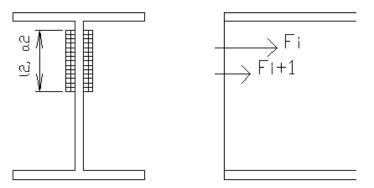
For all possible bolt groups, the maximum tension pro unit length is calculated. The tension pro unit length is  $(F_i + F_{i+1})/l2$ .
