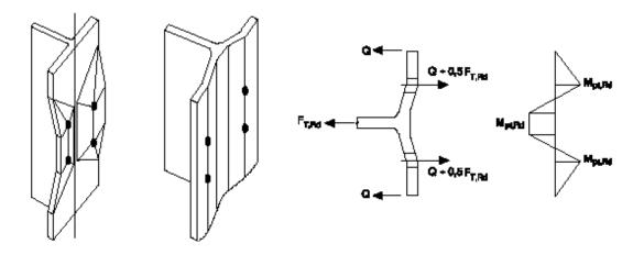
The bolts stay intact, only the column flange (or end plate) will yield.
