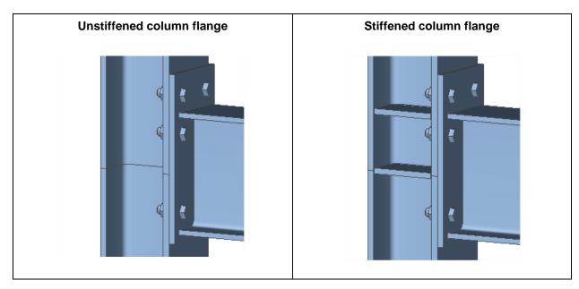
In this case the column flange is unstiffened. In the table below the difference is shown:
