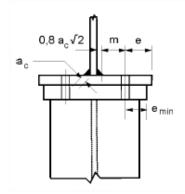
$\begin{array}{l} n = e_{min} = 40 \text{mm} \\ \leq 1,25 \cdot m = 1,25 \cdot 24,34 = 30,42 mm \\ \boldsymbol{n} = \boldsymbol{30}, \boldsymbol{42mm} \\ \text{w} = 80 \text{ mm} \end{array}$
