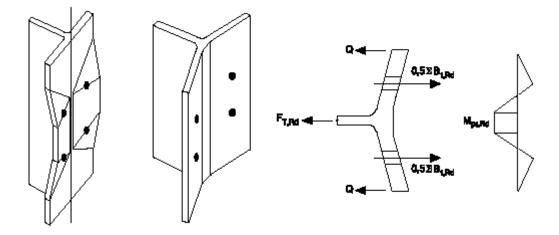
The bolts brake together with the yielding of the column flange (or end plate).
