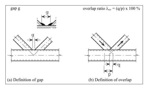
Either gap or overlap is calculated automatically by default using the structural model geometry and the value is shown in the properties of the joint object with reference to identified brace members. The
