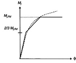
At the same time, a non-linear function is generated, representing the moment-rotation diagram.
