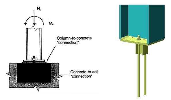
For more info about base plate design (shear irons, etc...), we refer to Ref.[2]. An example of a base plate connection in SCIA Engineer is given in **Example CON\_005.esa**, **Node N9**.
